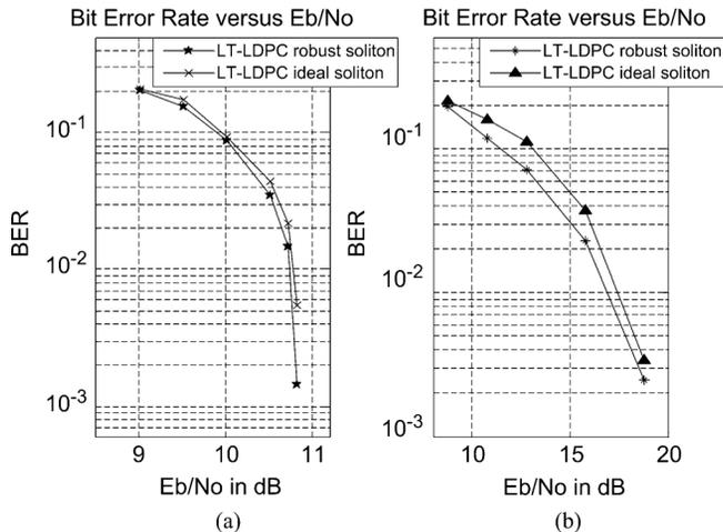
Fig. 5. BER versus  $E_b/N_0$  for concatenated LT and LDPC codes, with LT as the outer scheme (a) with and (b) without the method of treating packets as erasures at the decoding procedure.
