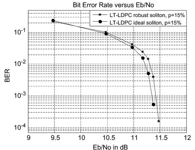
Fig. 6. BER versus  $E_b/N_0$  for concatenated LT and LDPC codes, with LT as the outer scheme with the proposed method, and with  $p = 15\%$  of transmitted packets affected by impulsive noise.
