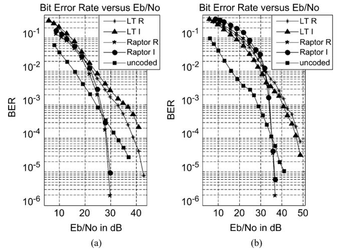
Fig. 2. BER versus  $E_b/N_0$  for LT and Raptor codes (LDPC and LT codes) with the ideal (LT I, Raptor I) and the robust soliton distribution (LT R, Raptor R), noise. (a) 10 dB stronger than  $N_0$ . (b) 20 dB stronger than  $N_0$ .
