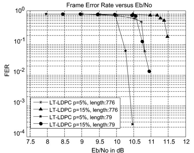
Fig. 9. FER versus  $E_b/N_0$  for concatenated LT and LDPC codes, with LT as the outer scheme with the proposed method.  $p = 5\%$  and  $p = 15\%$  of packets affected by impulsive noise.
