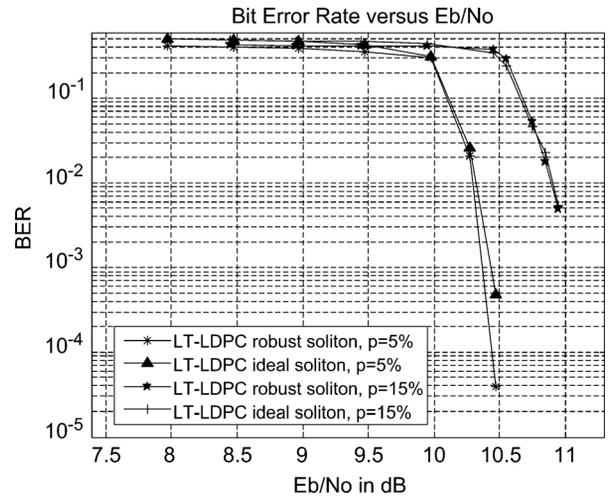
Fig. 8. BER versus  $E_b/N_0$  for concatenated LT and LDPC codes, with LT as the outer scheme with the proposed method.  $p = 5\%$  and  $p = 15\%$  of transmitted packets affected by impulsive noise, LT packet size: 79 b.
