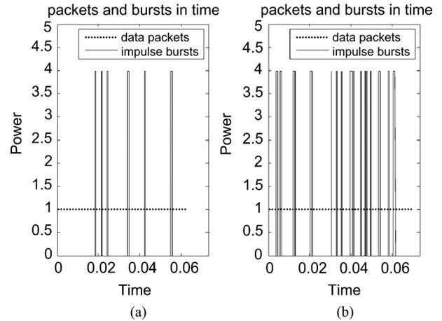
Fig. 4. Packet transmission and impulse bursts in time with (a)  $p = 5\%$  and (b)  $p = 15\%$  of packets affected by impulsive noise, respectively.
