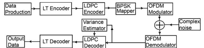
Fig. 3. System block diagram.
