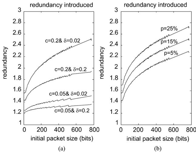
Fig. 7. Redundancy introduced to the proposed concatenated coding scheme by LT encoding in terms of the LT packet size. (a) For different values of  $c$  and  $\delta$ . (b) For a different percentage of packets affected by impulsive noise.
