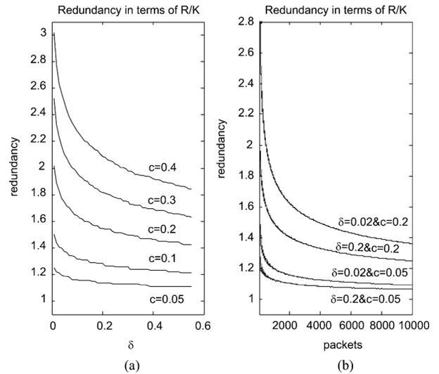
Fig. 1. Redundancy ( $red = R/K$ ) introduced by LT and Raptor codes for (a) different values of  $c$  and  $\delta$ , with  $K = 650$  and (b) for different values of  $K$  with fixed  $c$  and  $\delta$ .
