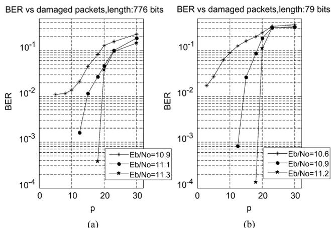
Fig. 10. BER versus the percentage  $p$  of damaged packets for fixed values of  $E_b/N_0$ . (a) Packet length: 776 bits. (b) Packet length: 79 bits.
