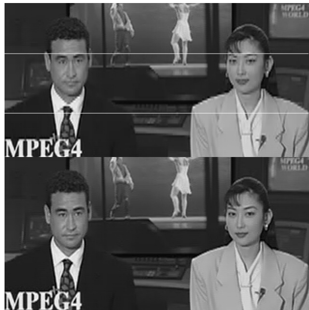
Fig. 5. Details of reconstructed frames for the two description MD system (top) and the frame-based MD system (bottom).
