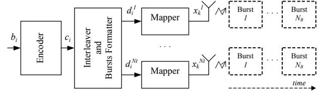
Fig.1. Bit-interleaved space-time coded transmitter.
