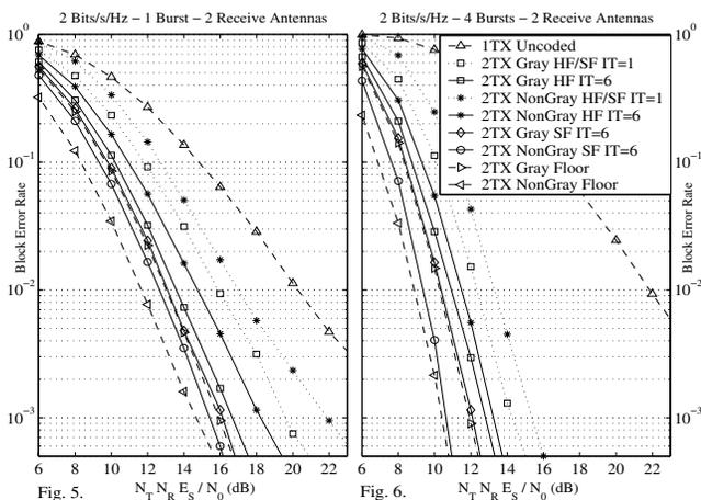
As in Fig. 3 and Fig. 4, with: double receive diversity, both Gray and Non Gray mapping, up to six decoding passes for both soft and hard feedback.
