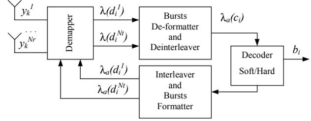
Fig.2. Iterative decoder. Feedback from the decoder can be soft or hard.
