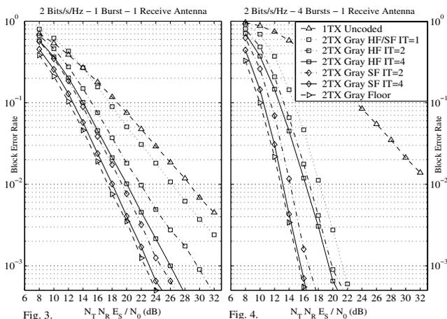
Block error rate versus average signal to noise ratio with double transmit and single receive diversity for transmission at 2 Bits/s/Hz of blocks of 240 information bits over one burst (Fig.3) or four independently faded bursts (Fig.4). Coding schemes of Table 1 with Gray mapping. Up to four decoding passes for both soft (SF) and hard (HF) feedback.
