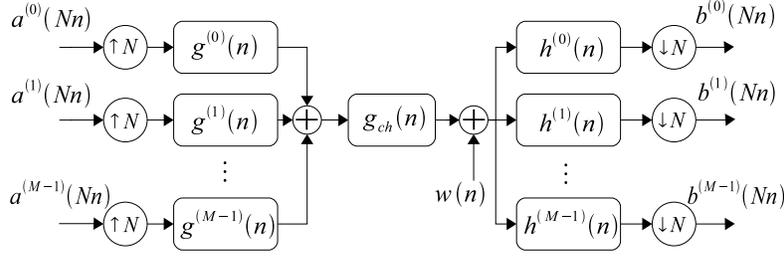
Fig. 1. General filter bank architecture.
