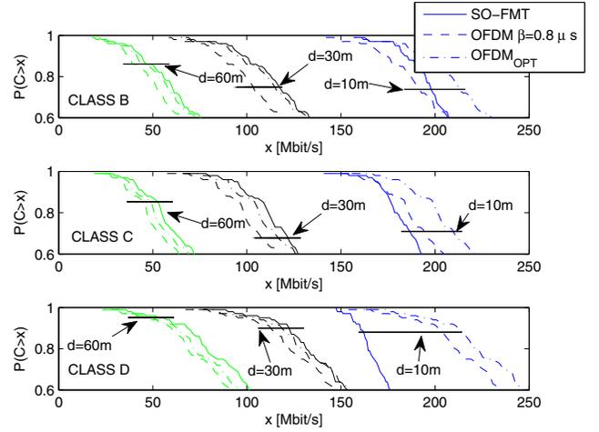
Fig. 3. Achievable rate CCDF obtained using SO-FMT, A-OFDM, and OFDM with a fixed CP of  $0.8 \mu\text{s}$ . The employed channel classes are the B, C, and D. The distance between transmitter and receiver is set to  $10 \text{ m}$ ,  $30 \text{ m}$ , and  $60 \text{ m}$ .
