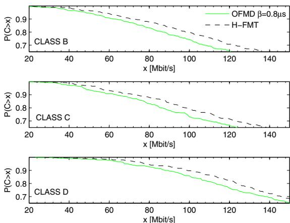
Fig. 5. Achievable rate CCDF using H-FMT and OFDM with fixed CP equal to  $0.8 \mu s$  for channel class B, C, and D.
