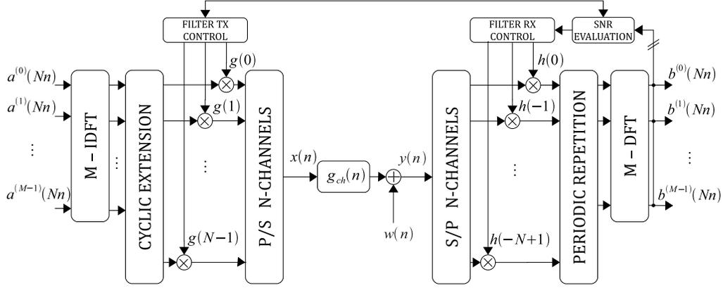
Fig. 2. Hybrid FMT scheme.
