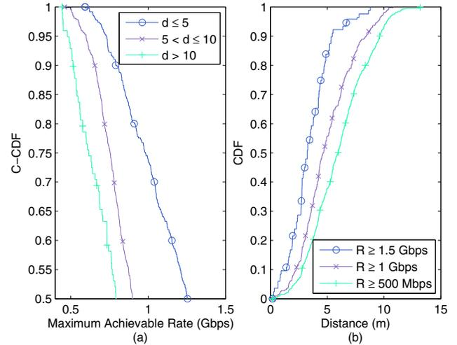
Fig. 6. On the left, complementary cumulative distribution function (C-CDF) of the maximum achievable rate for different ranges of distance. On the right, C-CDF of the distance for different values of achievable rate.
