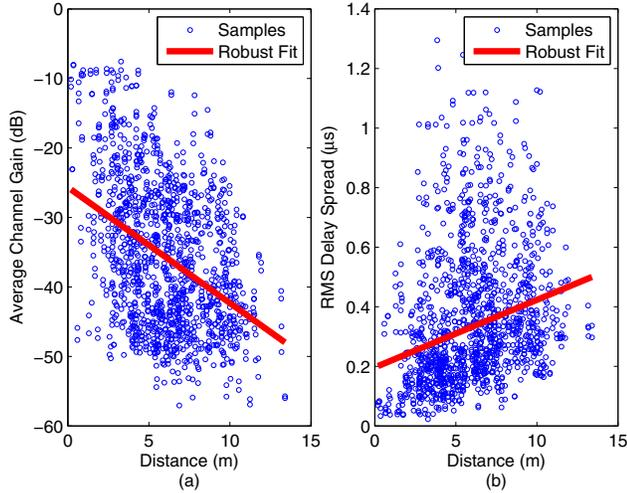
Fig. 4. On the left, average channel gain as a function of distance. On the right, RMS delay spread as a function of distance. In both cases, the linear robust fit is provided.
