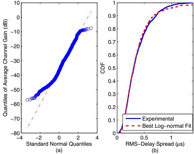
Fig. 2. On the left, quantiles of the average channel gain in dB versus the standard normal quantiles. On the right, cumulative distribution function of the RMS delay spread. The best log-normal fit is also shown.
