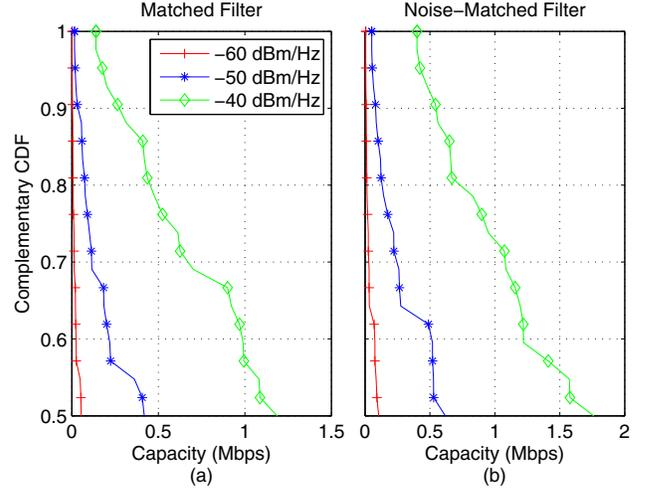
Fig. 7. Complementary CDF of the capacity for the matched filter receiver and noise-matched filter receiver on the left and the right, respectively. The results for three values of transmitted PSD are shown.
