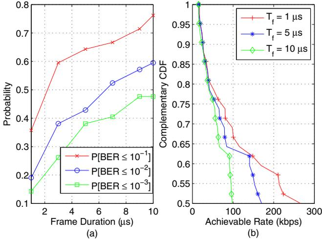
Fig. 9. CDF of the fixed BER probability and complementary CDF of the achievable rate as a function of the frame duration when the N-MF receiver is deployed on the left and the right, respectively.
