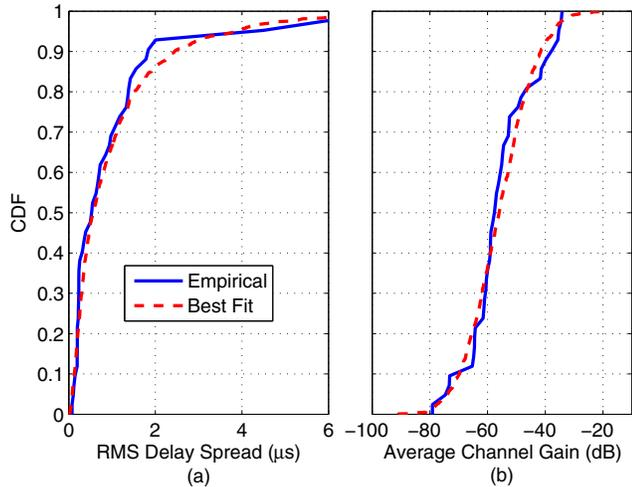
Fig. 3. On the left, CDF of the RMS-DS and its fit. On the right, CDF of the ACG in dB and its fit.
