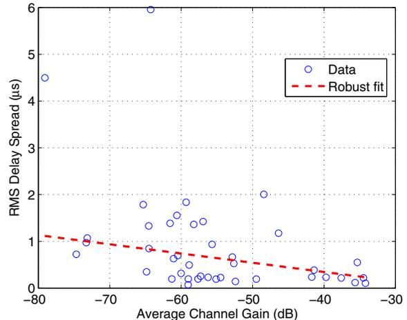
Fig. 4. RMS delay spread as a function of the ACG and its robust regression.
