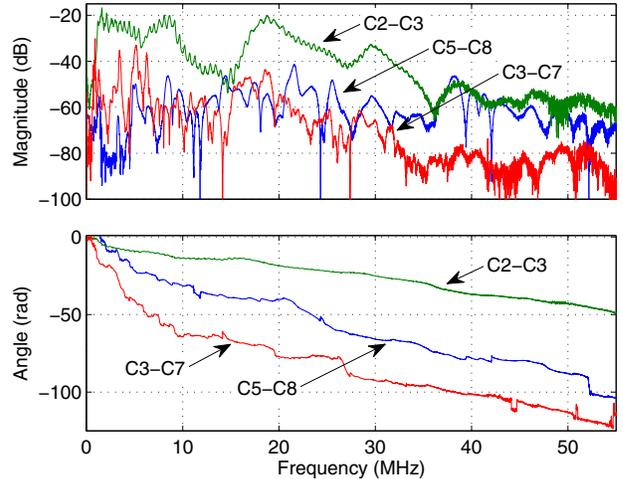
Fig. 2. Magnitude and phase of the frequency response of three different channels extracted from the MV test network.
