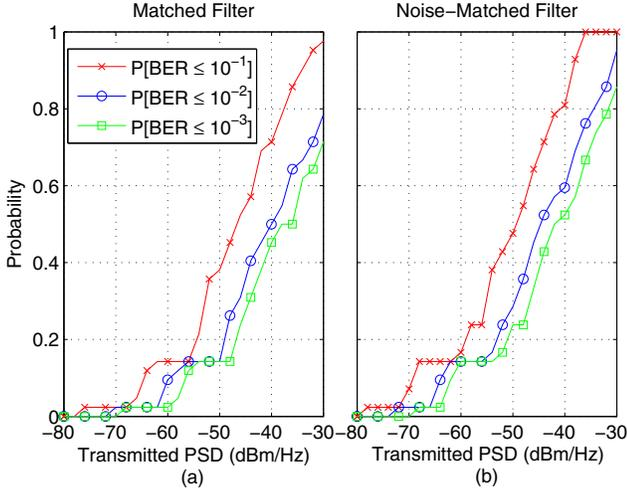
Fig. 5. CDF of the fixed BER probability for the matched filter receiver and the noise-matched filter receiver as a function of the transmitted PSD on the left and the right, respectively.
