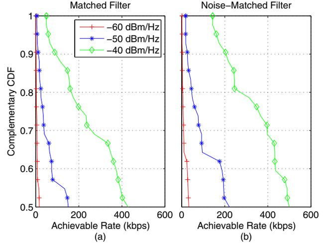
Fig. 6. Complementary CDF of the achievable rate (with hard decoding) for the matched filter receiver and noise-matched filter receiver on the left and the right, respectively. The results for three values of transmitted PSD are shown.
