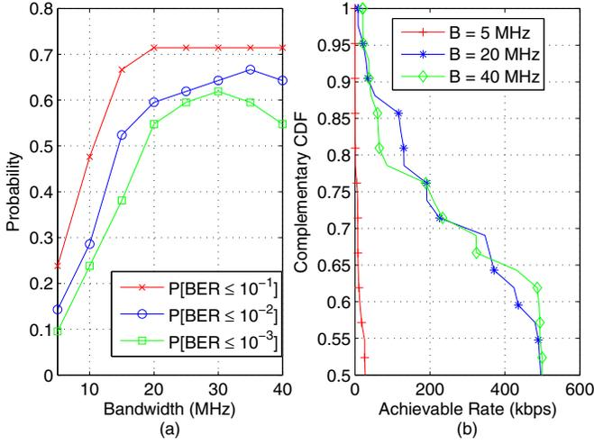
Fig. 8. CDF of the fixed BER probability and complementary CDF of the achievable rate as a function of the pulse bandwidth when the N-MF receiver is deployed on the left and the right, respectively.
