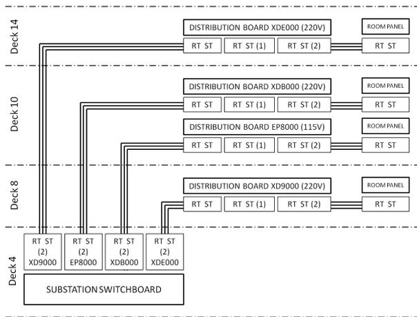
Fig. 1. Measurement scenario. RT and ST denotes test points with a coupler connected to R and T phases or between S and T phases. RT ST, RT ST (1) and RT ST (2) denote respectively test points at the input of the primary circuit breaker, at the output of it, and at the output of the secondary circuit breaker, respectively.
