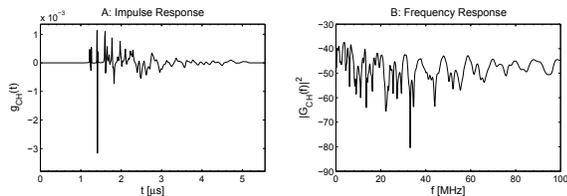
Fig. 2. Realization of PLC channel impulse response and frequency response.
