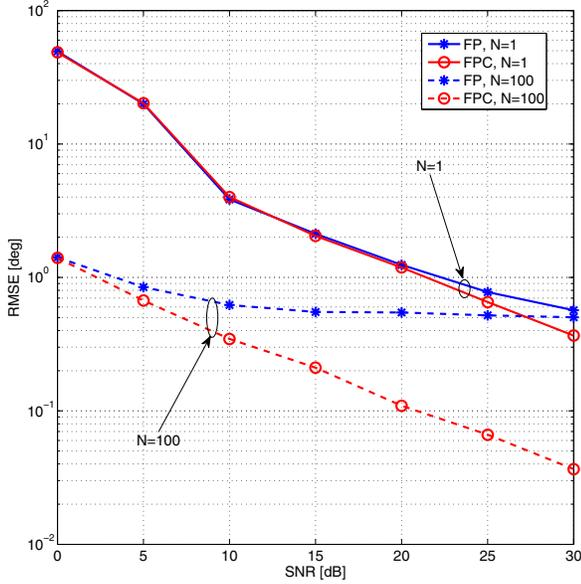
Fig. 5. Comparison between full-parallel architecture with incoherent (FP) and coherent (FPC) LOs. Performance results are obtained by using the root-MUSIC algorithm with  $M = 4$  antennas and  $N = \{1, 100\}$  samples.
