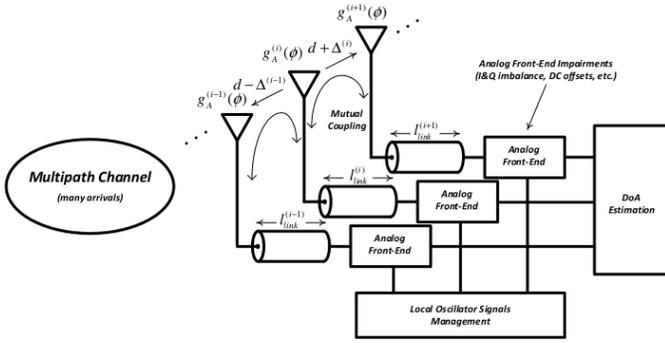
Fig. 2. System model for DoA estimation with typical error sources.
