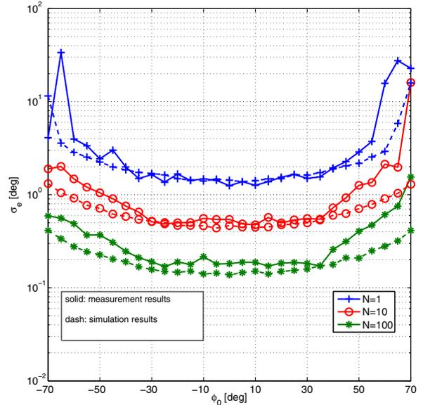
Fig. 4. Simulated and experimental results as a function of the DoA  $\phi_0$  and the number of samples  $N$  with root-MUSIC algorithm. SNR= 13 dB.
