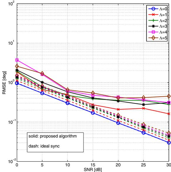
Fig. 3. RMSE of the DoA estimator in [15] as a function of both the receiver SNR and the MP Poisson arrival process mean  $\Lambda$ .
