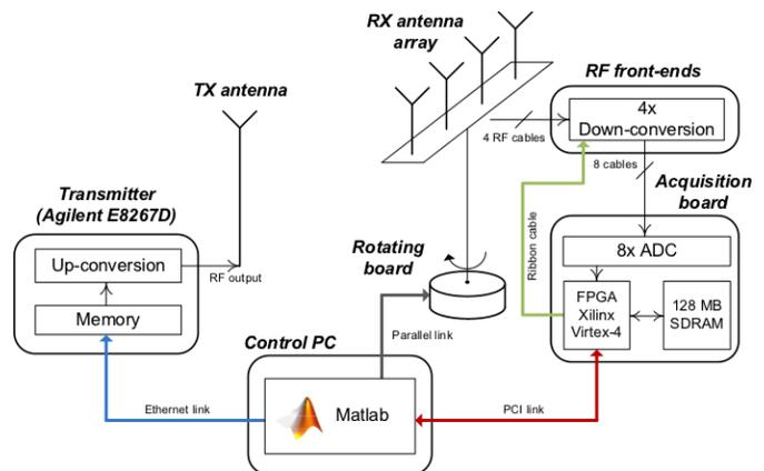
Fig. 1. SIMO wireless testbed developed at the WiPLi Lab.
