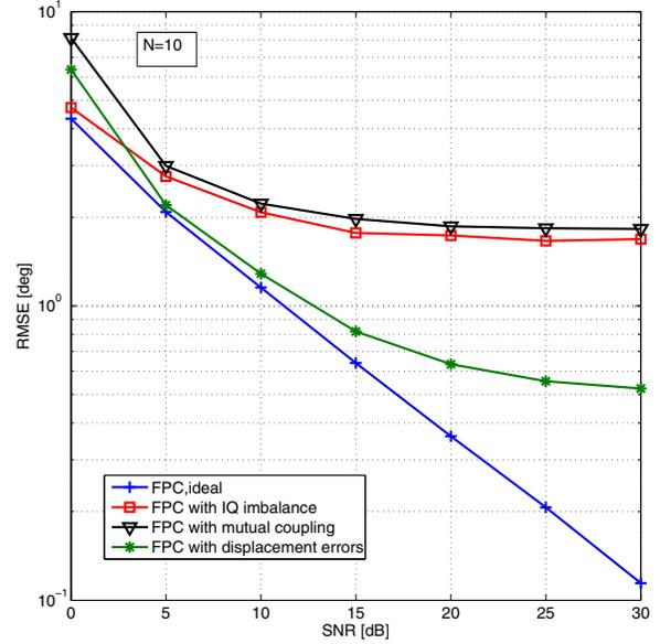
Fig. 6. Comparison among the effect of non idealities in a full-parallel architecture with coherent LOs (FPC). Performance results are obtained by using root-MUSIC algorithm with  $M = 4$  antennas and  $N = 10$  samples.
