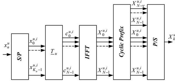
Figure 1. Baseband DMT-OFDMA transmitter of user  $u$ .
