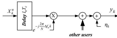
Figure 2. Baseband equivalent channel model for user  $u$ .
