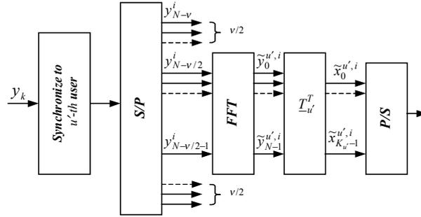
Figure 3. Baseband DMT-OFDMA receiver synchronized to user  $u'$ .
