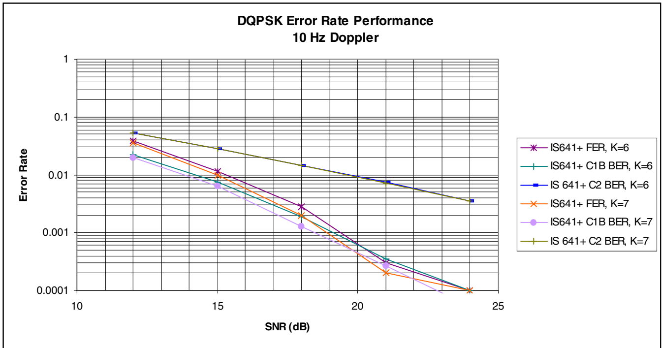
Figure 5. IS641+ Error Rate Performance at 10 Hz Doppler Comparing K=6 with K=7.
