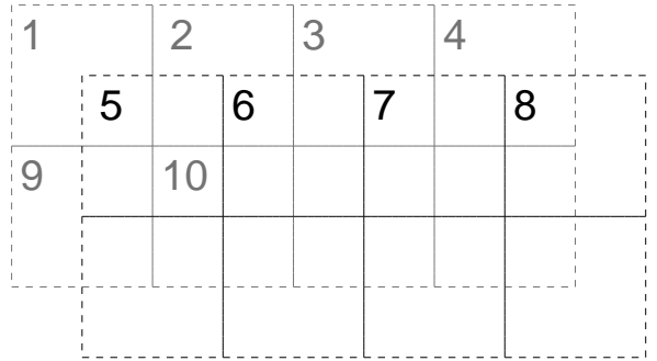
Fig. 3. Ordering used for sending the coefficients in our experiment. Numbers in the blocks show the order the block coefficients are sent.
