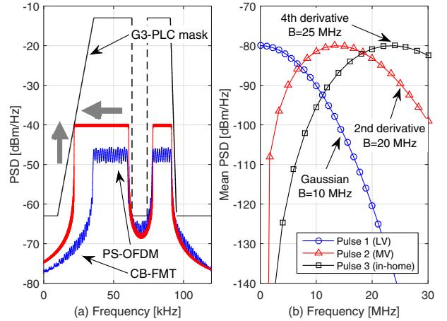
Fig. 8. PSD in CENELEC-A band for PS-OFDM and CB-FMT (a) and mean PSD of transmitted UWB pulses for LV, MV and in-home scenarios (b).
