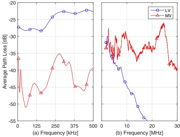
Fig. 2. Average path loss profile for outdoor LV and MV lines in both the NB (a) and BB (b) frequency range.
