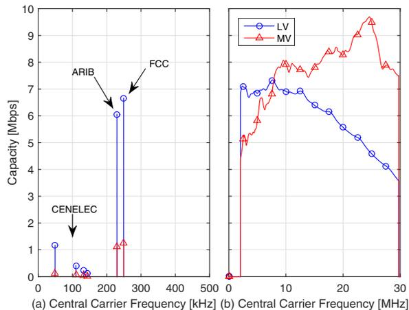
Fig. 7. Capacity for LV and MV scenarios in the NB (a) and BB (b) frequency range. For the BB case a bandwidth of 500 kHz is considered.
