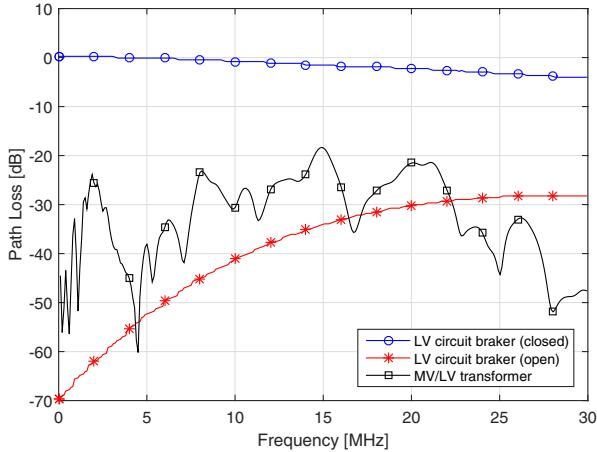
Fig. 4. Path loss of a LV circuit breaker, for both open and closed configurations, and of a bypass ML/LV transformer along frequency.
