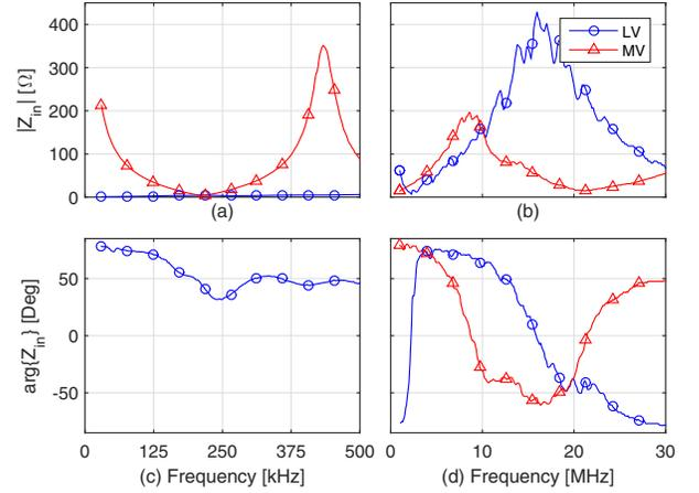
Fig. 3. Magnitude (on top) and phase (on bottom) of the input impedance for outdoor LV and MV lines in the NB (left side) and BB (right side) range.
