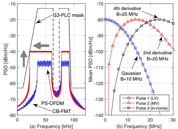
Fig. 8. PSD in CENELEC-A band for PS-OFDM and CB-FMT (a) and mean PSD of transmitted UWB pulses for LV, MV and in-home scenarios (b).
