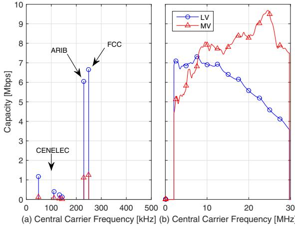
Fig. 7. Capacity for LV and MV scenarios in the NB (a) and BB (b) frequency range. For the BB case a bandwidth of 500 kHz is considered.
