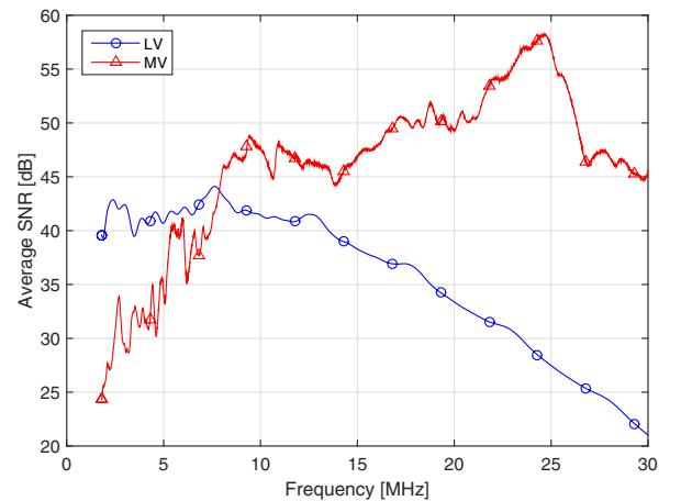
Fig. 6. SNR trend for LV and MV scenarios in the BB frequency range.
