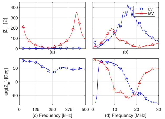
Fig. 3. Magnitude (on top) and phase (on bottom) of the input impedance for outdoor LV and MV lines in the NB (left side) and BB (right side) range.
