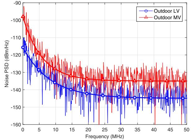
Fig. 5. LV and MV background noises. The exponential model is also shown.
