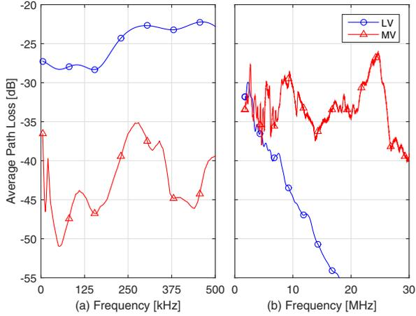
Fig. 2. Average path loss profile for outdoor LV and MV lines in both the NB (a) and BB (b) frequency range.
