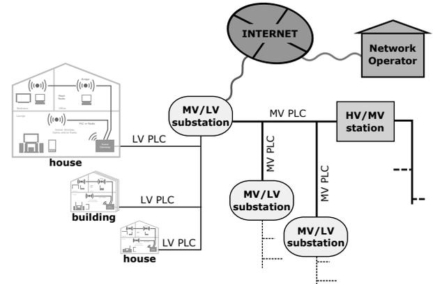
Fig. 1. Schematic of a typical power distribution grid.
