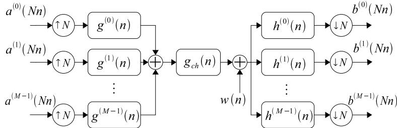
Fig. 1. General filter bank architecture.
