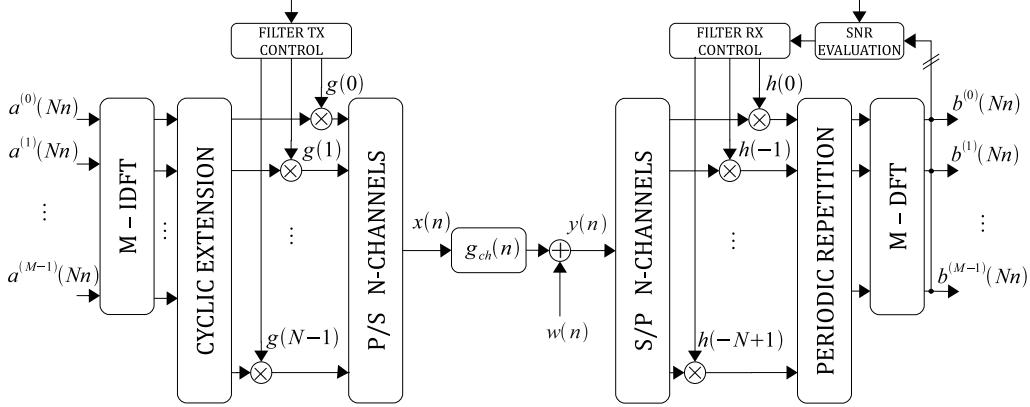
Fig. 2. Hybrid FMT scheme.
