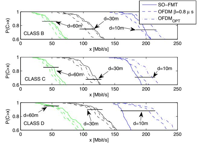
Fig. 3. Achievable rate CCDF obtained using SO-FMT, A-OFDM, and OFDM with a fixed CP of  $0.8 \mu\text{s}$ . The employed channel classes are the B,C, and D. The distance between transmitter and receiver is set to 10 m, 30 m, and 60 m.
