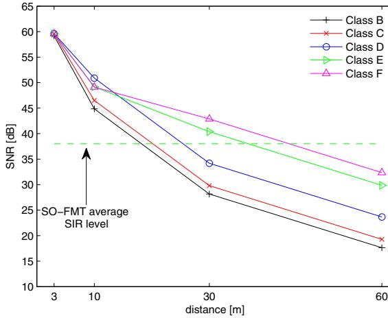
Fig. 4. SNR as function of the distance, and mean value of SIR for the SO-FMT.
