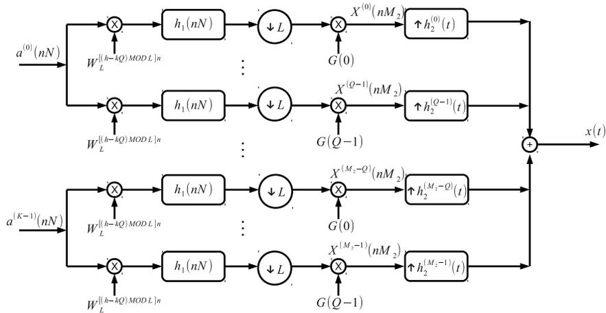
Fig. 3. Linear equivalent model for CB-FMT transmitter.
