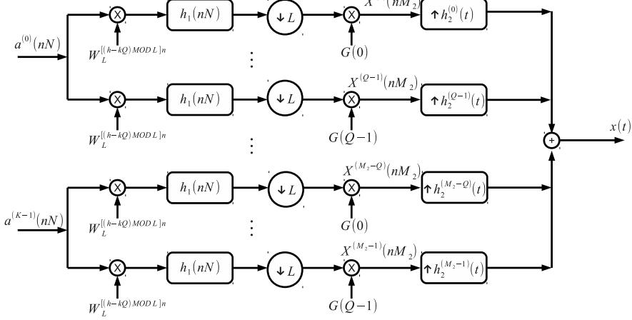
Fig. 3. Linear equivalent model for CB-FMT transmitter.
