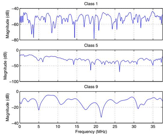
Fig. 5. Magnitude of three channel realizations generated with the statistical top-down model.
