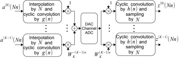
Fig. 1. CB-FMT transceiver scheme.
