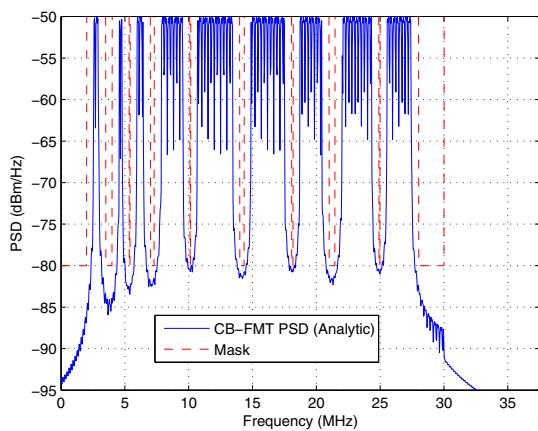
Fig. 4. Power Spectral Density of CB-FMT transmitted signal and the HomePlug notching mask.
