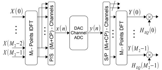
Fig. 2. Outer cyclic extension with frequency domain equalizer.
