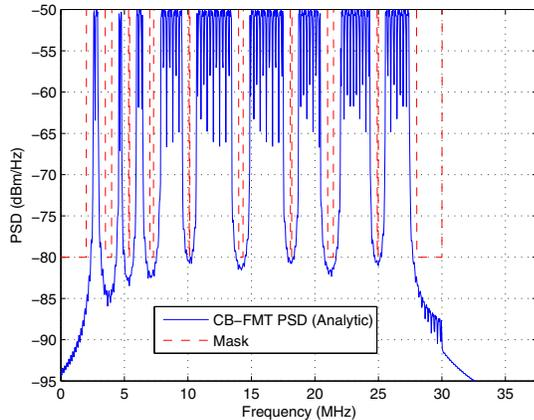
Fig. 4. Power Spectral Density of CB-FMT transmitted signal and the HomePlug notching mask.
