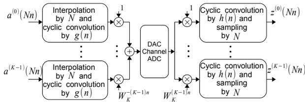
Fig. 1. CB-FMT transceiver scheme.
