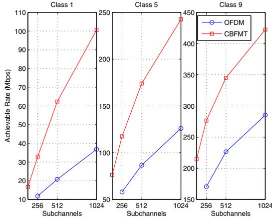
Fig. 6. Achievable rate for CB-FMT and OFDM as a function of sub-channel number.
