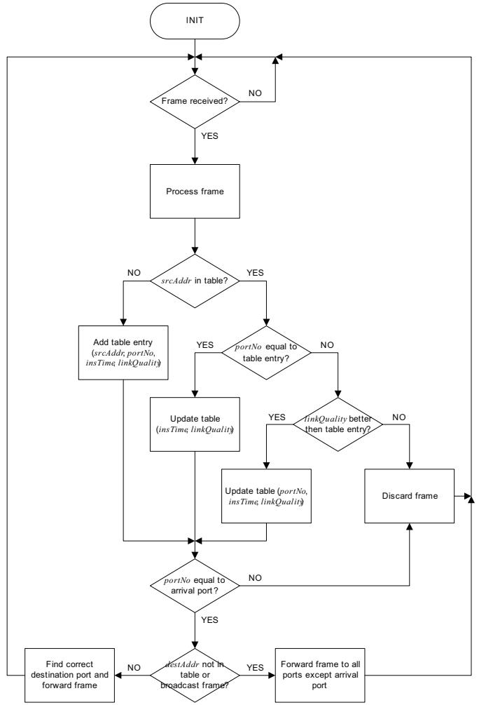
Fig. 4. Switch flow chart.
