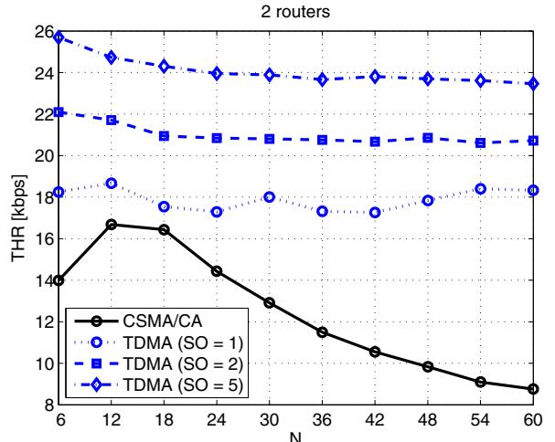
Fig. 8. Aggregate throughput comparison between CSMA/CA and TDMA for a network configuration with 2 routers.
