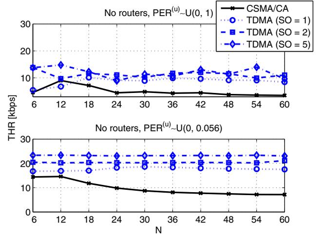
Fig. 7. Aggregate throughput comparison between CSMA/CA and TDMA for a network configuration without routers.
