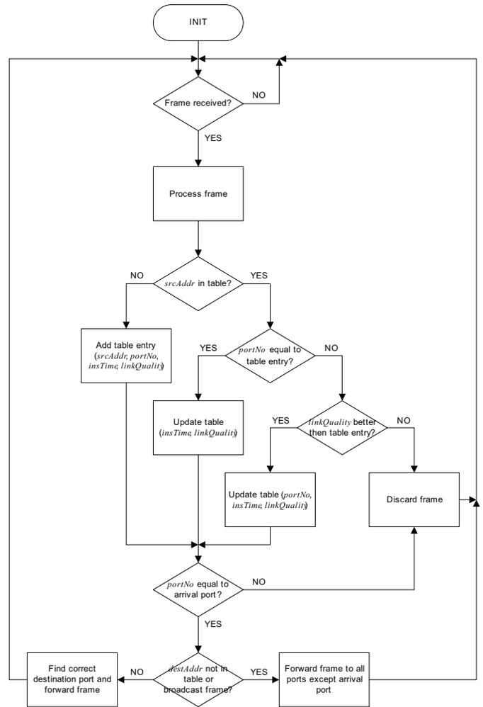
Fig. 4. Switch flow chart.
