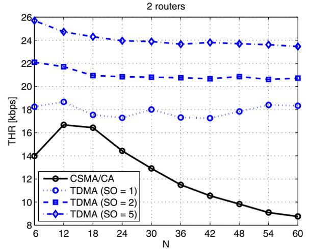
Fig. 8. Aggregate throughput comparison between CSMA/CA and TDMA for a network configuration with 2 routers.
