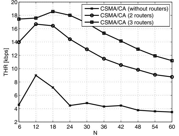
Fig. 5. Aggregate throughput according to different network configurations using CSMA/CA.
