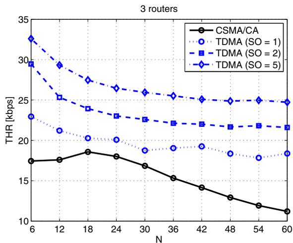
Fig. 9. Aggregate throughput comparison between CSMA/CA and TDMA for a network configuration with 3 routers.
