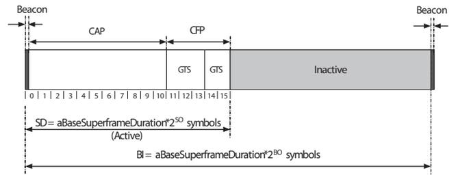
Fig. 6. An example of superframe structure for the beacon-enabled mode of the IEEE 802.15.4.
