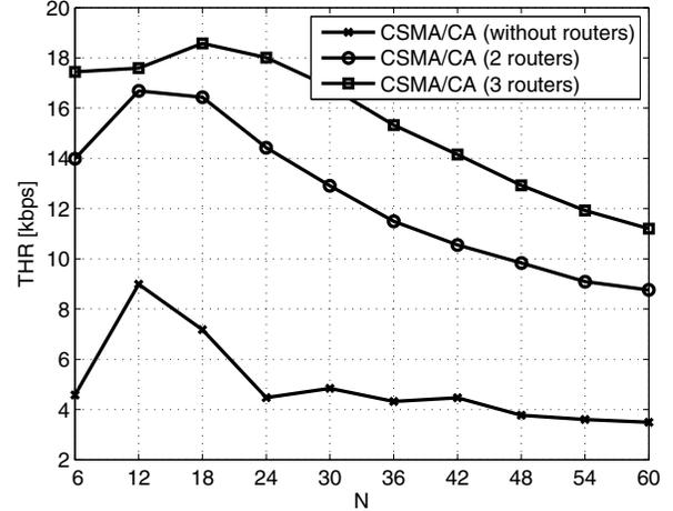
Fig. 5. Aggregate throughput according to different network configurations using CSMA/CA.
