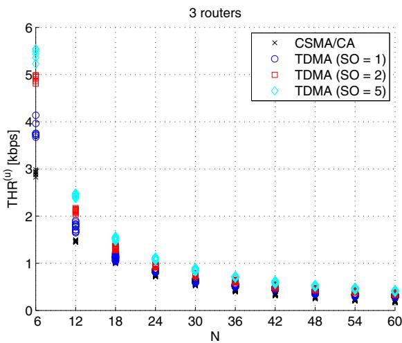
Fig. 10. Throughput achieved by each node in a 3 routers network using CSMA/CA or TDMA.
