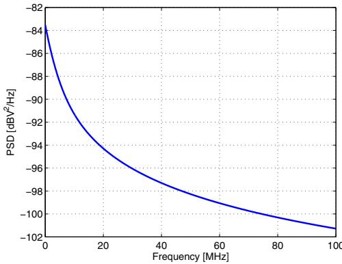
Fig. 6. Impulsive noise PSD profile at the receiver side for  $N_I = 5$ .
