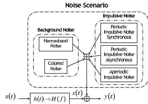
Fig. 1. Noise scenario on power line communications.
