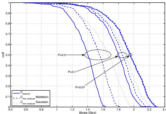
Fig. 7. Channel efficiency with different coding techniques combined with the proposed noise model.
