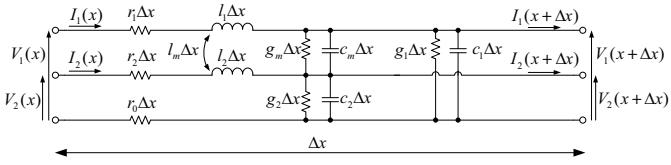
Fig. 1. Equivalent per-unit-length representation of a section of three conductors line.
