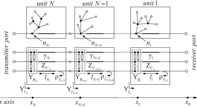
Fig. 2. On the top, unifilar description of the remapped topology. On the bottom, the correspondent representation in units.
