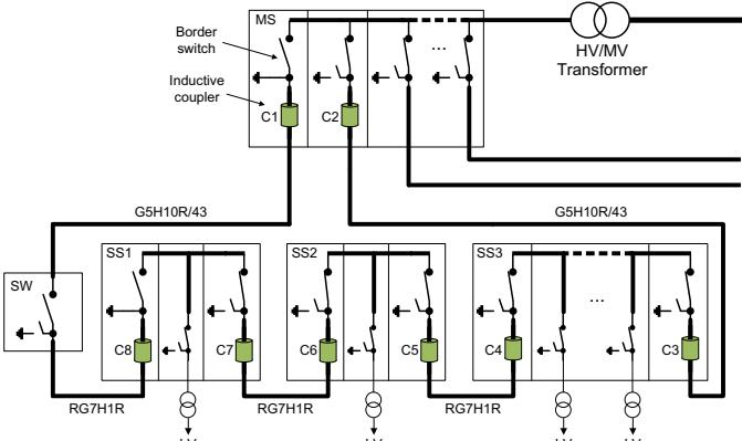
Fig. 1. Layout of the MV test network.
