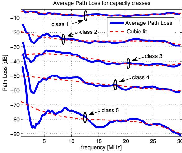
Figure 5. Average path loss profiles and their cubic fit for each class of capacity.
