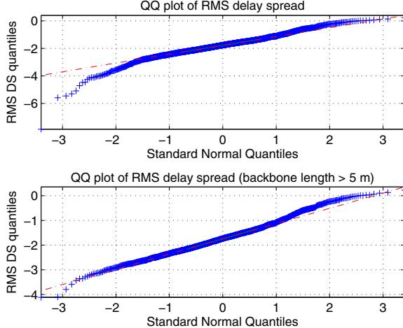
Figure 3. Quantiles of  $\bar{\sigma}_\tau$  (in the top plot) and  $\hat{\sigma}_\tau$  (in the bottom plot) versus standard normal quantiles.
