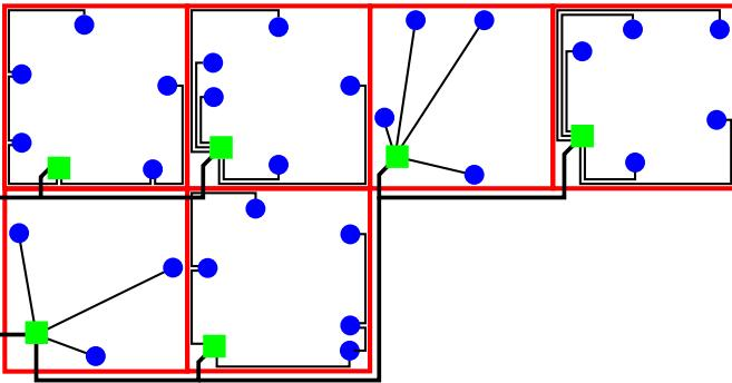
Figure 1. An example of topology arrangement generated by the algorithm. Derivation boxes and outlets are represented by the squared and dotted markers, respectively.
