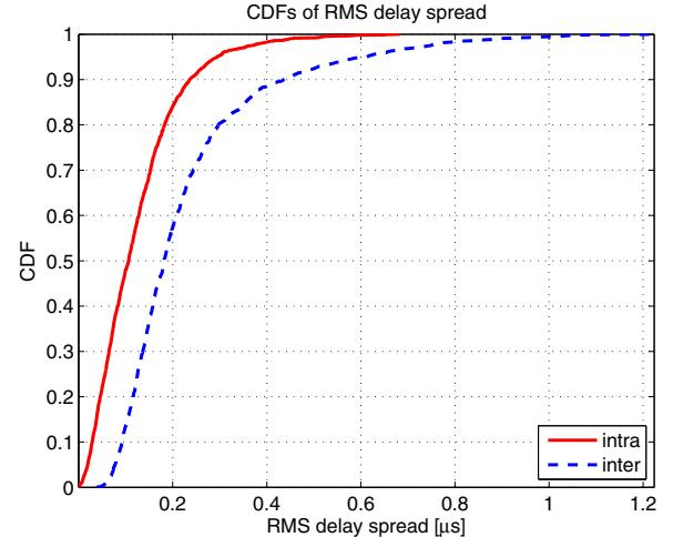
Figure 7. Cumulative distribution functions of RMS delay spread for intracluster and intercluster classes.
