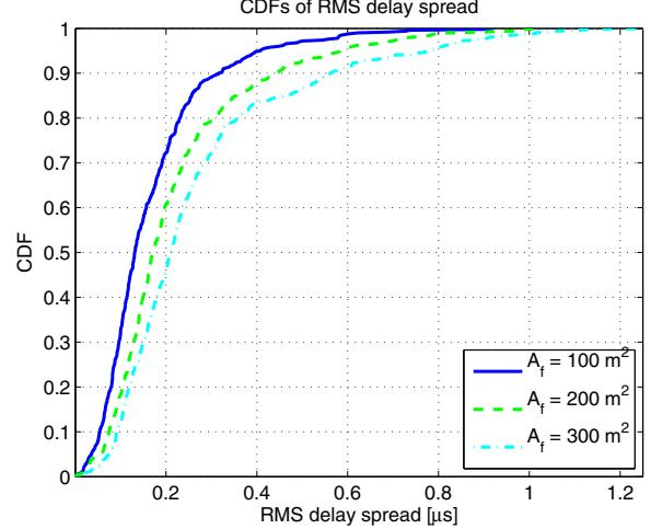
Figure 2. Cumulative distribution functions of the RMS delay spread as a function of the topology area  $A_f$ .
