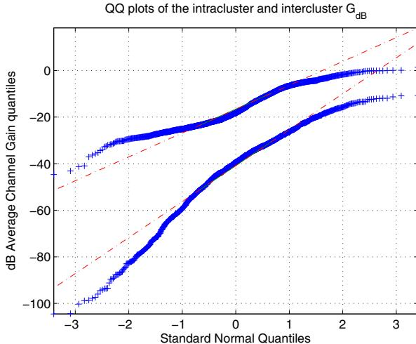
Figure 8. Quantiles of the intercluster and intracluster average channel gain in dB versus standard normal quantiles.
