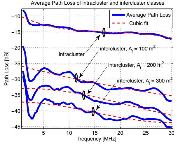
Figure 6. Average path loss profiles and their cubic fit for the intracluster and intercluster classes.
