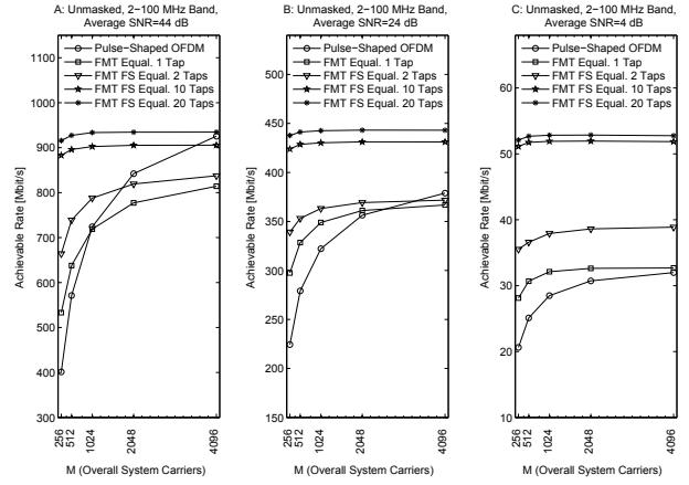
Fig. 5. Achievable rate comparison. Unmasked case in the 2-100 MHz band.
