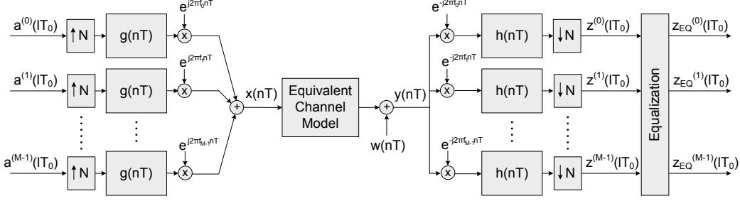
Fig. 1. General scheme for a filter bank based system.
