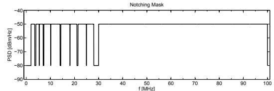
Fig. 4. PSD mask in the 0-100 MHz band.
