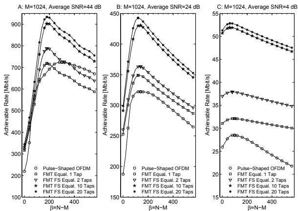
Fig. 3. Achievable rate as a function of the system overhead  $\beta$ .
