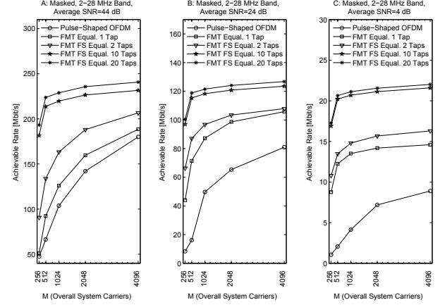
Fig. 7. Achievable rate comparison. Masked case in the 2-28 MHz band.
