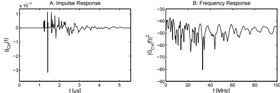
Fig. 2. Realization of PLC channel impulse response and frequency response.
