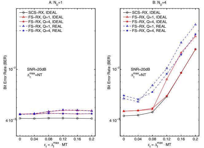
Fig. 4. Average BER as a function of the maximum frequency offset for 1 user and 4 users case. Ideal performance for SCS-RX and FS-RX. Practical performance for the FS-RX.
