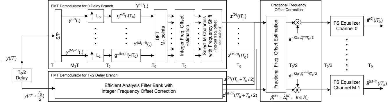
Fig. 2. Fractionally spaced multiuser receiver efficient implementation.
