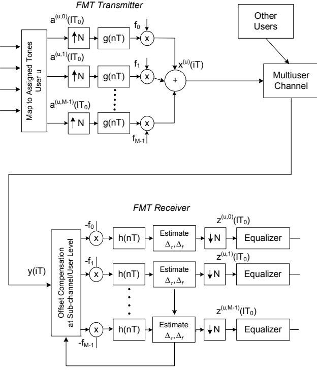
Fig. 1. Multiuser FMT system model with transmitter and receiver of user  $u$ .
