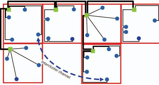
Figure 1. A typical in-home topology layout showing derivation boxes (square marker) and connections with outlets (dot markers).
