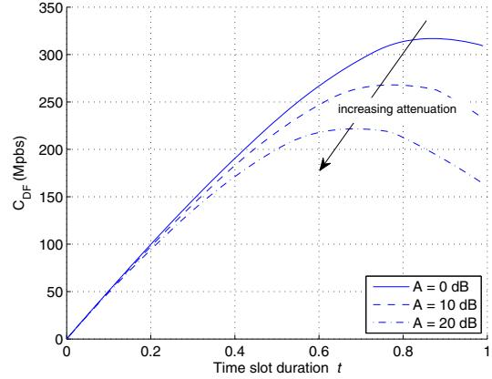
Figure 7. Average capacity  $C_{DF}(CB, t)$  for cross-breaker channels as a function of the time slot  $t$ .
