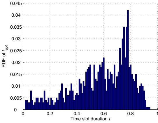
Figure 4. Probability density function of the optimal time slot allocation for the SDB configuration.
