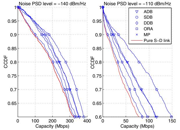
Figure 5. Complementary cumulative distribution function of capacity for different relay arrangements and for two noise levels.
