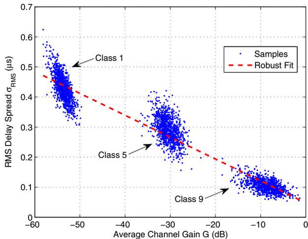
Fig. 3. Scatter plot of the RMS delay spread versus the average channel gain.
