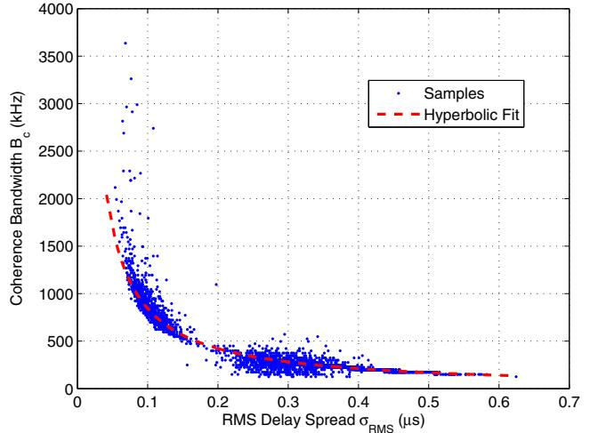
Fig. 4. Scatter plot of the coherence bandwidth versus the RMS delay spread.
