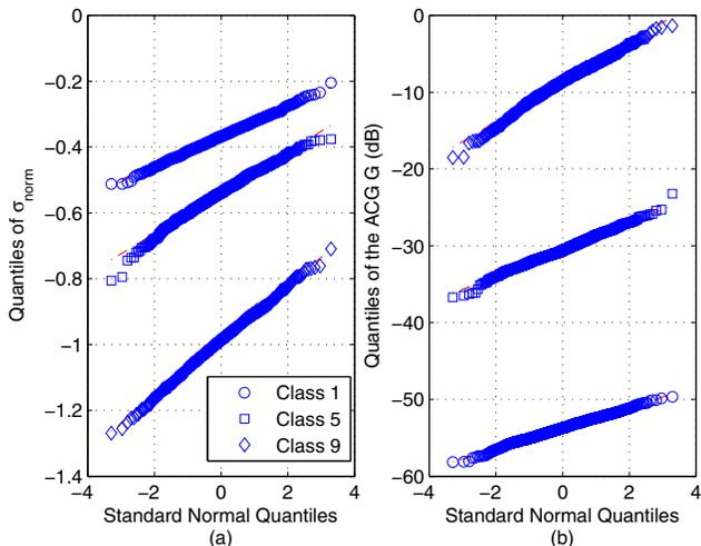
Fig. 2. On the left, QQ-plot of the normalized logarithmic delay spread ( $\sigma_{norm}$ ). On the right, QQ-plot of the average channel gain ( $G$ ).
