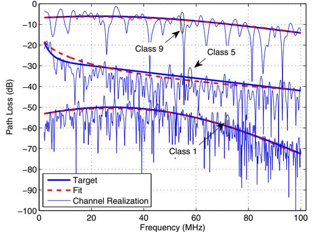
Fig. 1. Target path loss, fitted path loss and channel realizations of class 1 (bottom), class 5 (middle), and class 9 (top).
